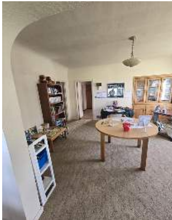
Photo 6: Texturing on walls and ceiling tested non-detect or less than 1% of asbestos (0.25%)
